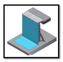
The proposed floor membrane will be our Evolution membrane, which is exclusive to Myrtha. Evolution is reinforced by fiberglass instead of polyester and therefore doesn't stretch and is further enhanced by the most chemically and UV resistant surface treatments available. The membrane will be mechanically fastened to the existing concrete. The result of which is a permanent fully adhered system that will not wrinkle or balloon under any circumstances.
